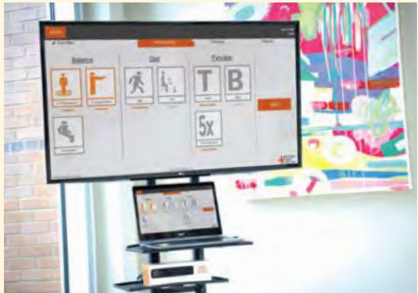
The VirtuSense system uses 3D motion analysis and biofeedback to precisely assess a person's balance, gait and function.
